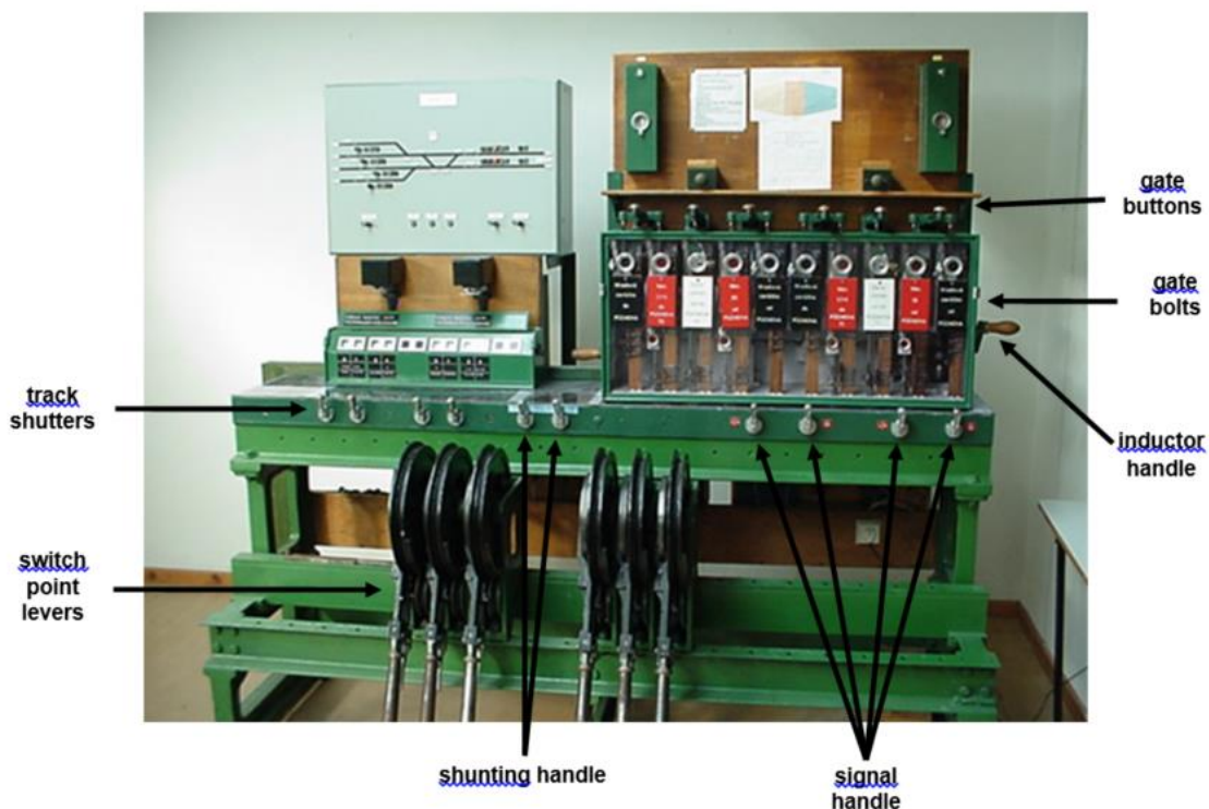
Figure 11 Control elements on the electromechanical safety device (signal interlocking box)
